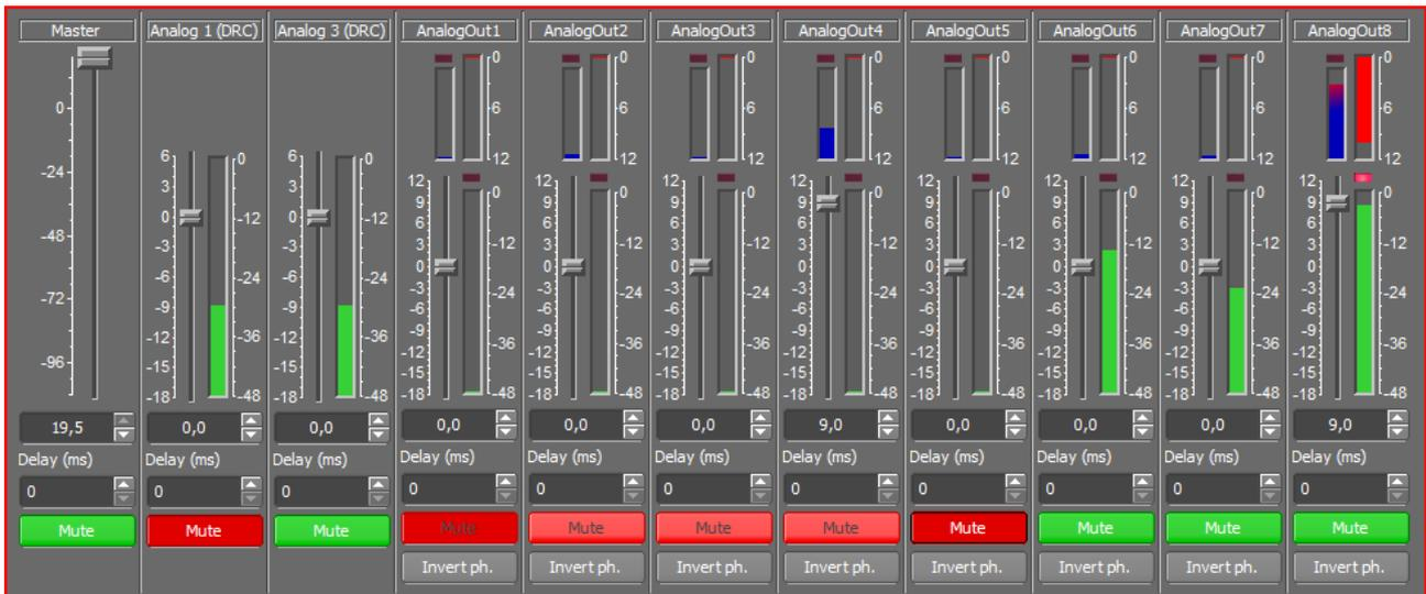
*Fig. 17: Example: Outputs AnalogOut1 and 5 are muted. Input Analog 1 (DRC) is muted → the mute buttons for AnalogOut1-4 are disabled. At AnalogOut1, it can be seen, that both, the output itself and the corresponding input are muted.*
